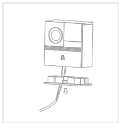
**Step 7:** Install the bottom door of the doorbell main unit and fix it with screws.
