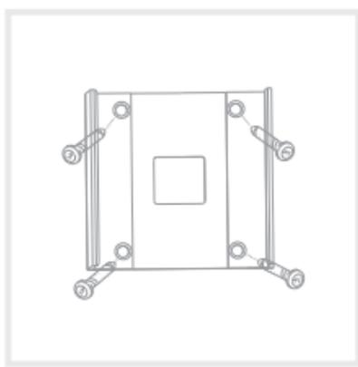
**Step 6:** Fix the mounting bracket to the wall.
