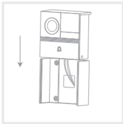
**Step 8:** Pull the power cable from the center hole of the bracket and slowly insert the doorbell into the door as shown in the above figure (be careful not to catch your finger).
