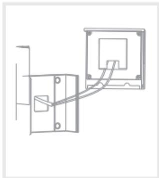
**Step 3:** Remove the double sided adhesive on the back of the mylar sheet. Cover the position of the power interface on the back of the doorbell host.
