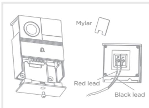
**Step 2:** Remove the bottom cover and bracket of the doorbell host and lead the output terminal. Connect to the power interface on the back of the doorbell host.
