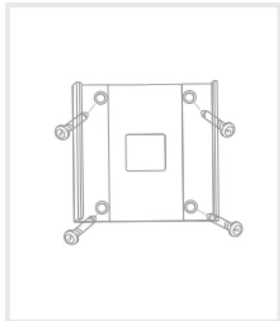
**Step 4:** Fix the mounting bracket to the wall.
