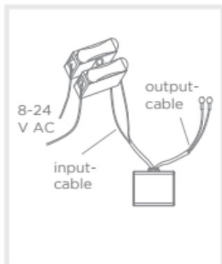
**Step 1:** Each input-cable (AC 8-24V) connect to the wires which come out of the wall.
