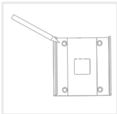
**Step 2:** Use the marker to draw 4 screw holes on the surface of the wall to be installed.
