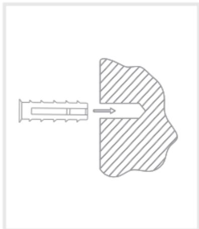
**Step 3:** Screw 4 expansion screws into the newly marked position.
