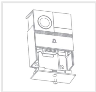
**Step 1:** Remove the doorbell bottom cover and bracket as shown in the figure.
