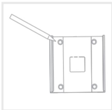
**Step 4:** Use the marker to draw the positions of the 4 screw holes on the wall surface to be installed.
