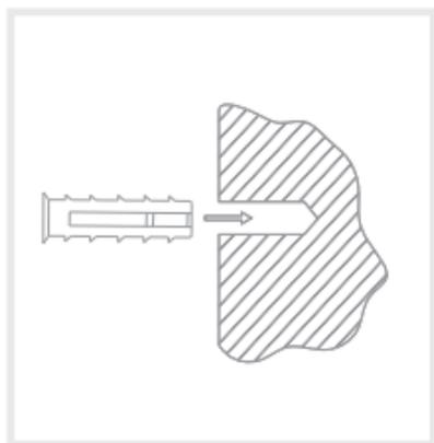
**Step 5:** Screw 4 expansion screws into the newly marked position.
