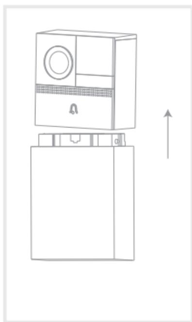
**Step 5:** Snap the doorbell into the bracket.
